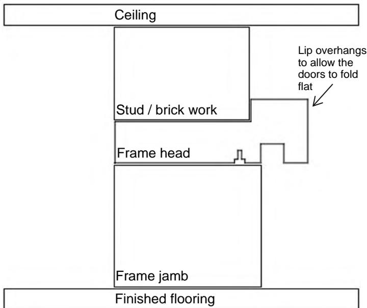
When you install the frame into your opening, the upstand on the frame head will wrap around the face of your stud / brickwork, as shown opposite.
