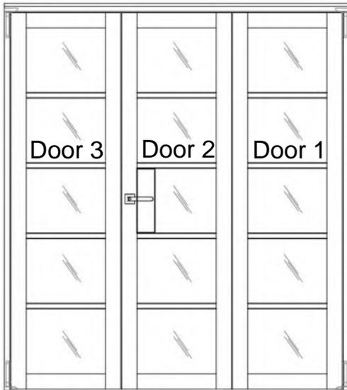
Fix the bottom pivot hinge plate **ONLY** onto the edge of the Pivot door, Door 1 using the torx screws provided and the 1/4 Hex T30 bit (E) into the predrilled holes.
