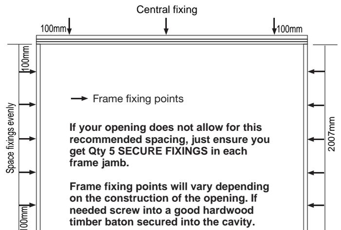
**Very important: Carefully check the frame is tightly fixed together and is square. Diagonals of the frame must be equal. Do not proceed with installation if the frame is not square.**
