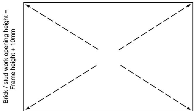
**Standard sized internal folding door sets outer frame dimensions are as follows;**
