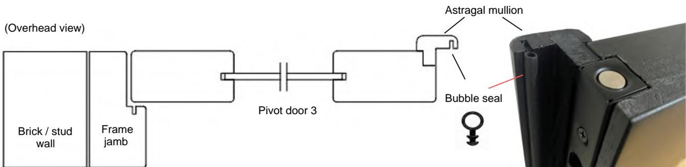
The astragal mullion has been piloted with screw holes, using the Qty 5 black pozi wood screws (L) provided and the Pozi No. 2 insert bit (I) provided, fix the astragal to the Pivot door, Door 3.
