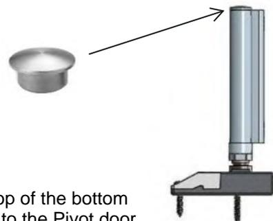
Fit the end cap to the top of the bottom pivot hinge barrel fixed to the Pivot door.
