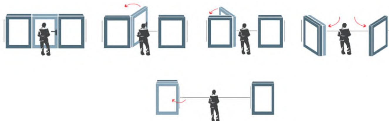
When closing the internal folding room divider door set, first close the Pivot door, Door 3, securing in place using the top and bottom finger operated bolts located on the side edge of the door.
