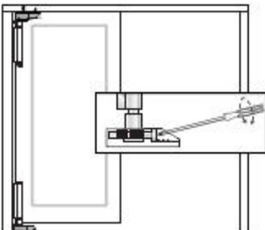
The opposite is the recommended spacing for our internal folding doors, however adjust the doors as required to achieve smooth operation.
