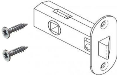
Fit the latch striker plate into the pre-machined position in the Pivot door, Door 3 using Qty 2 3/4" x 6s Pozi wood screw and Pozi No.2 bit (I) provided.
