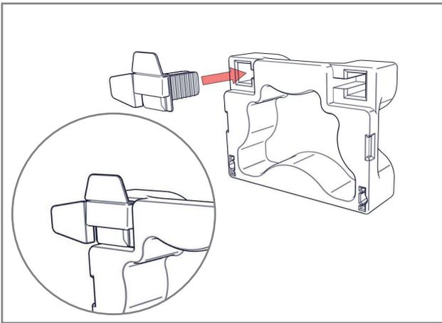
**1.** Place the top corner bracket into the top left slot on the bracket fitting tool.
