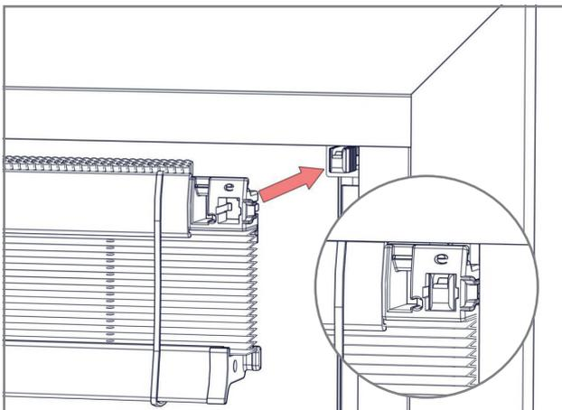
**15.** Align headrail endcaps with both top corner fixing brackets and push fully home. Your headrail should now be mounted to the frame.
