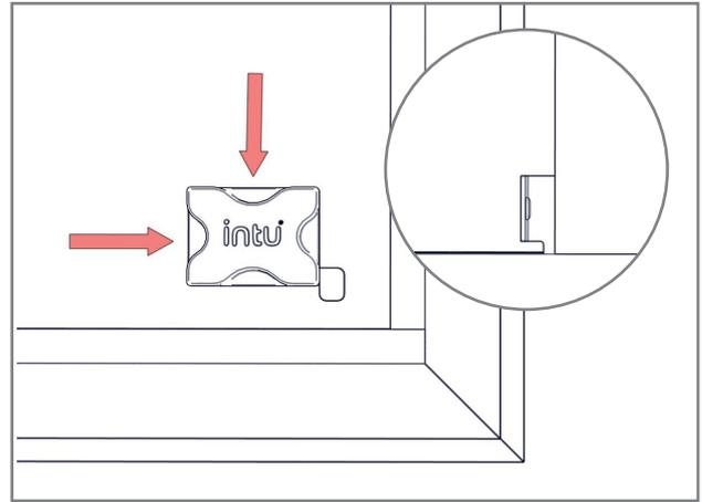
6. Position bracket behind the rubber seal at the bottom right corner of the frame. Carefully push until the metal leg is behind the rubber seal. Check the bracket is square to the sides of the frame and fully secure.
