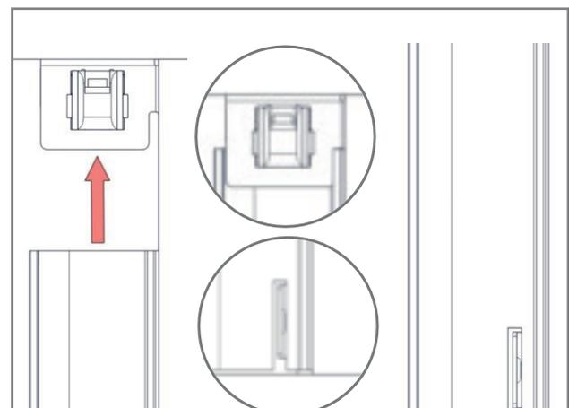
10. Slide the side extrusion up until its slots into the top corner fixing bracket. The side extrusion should rest under the bracket. Push the slot at the base of the extrusion over the bottom corner bracket. Repeat for both sides.
