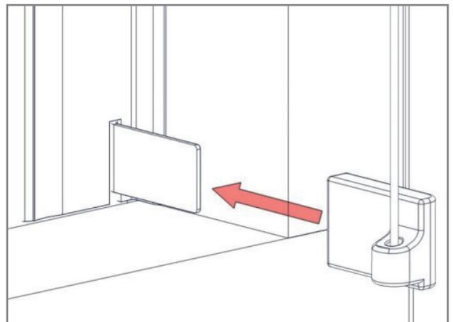
**16.** Align the bottom button with the bottom corner brackets. Slide the bottom button onto the bracket until it locates. Repeat for other side.
