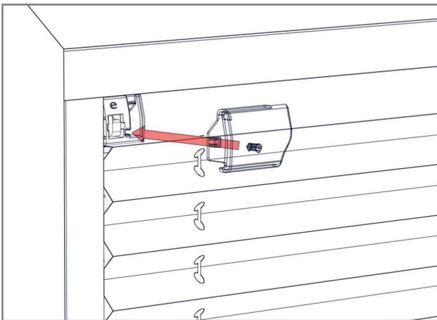
**19.** Re-attach the endcap covers by aligning the central post with the central hole on the endcap. Push the endcap cover in fully until a click is heard. Ensure the blind is lowered before doing this to prevent catching the fabric.
