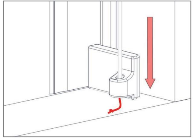
**18.** If your blind requires further tension, pull the cord through the hole in the bottom button until you feel the blind has sufficient tension and tie a fresh knot.
