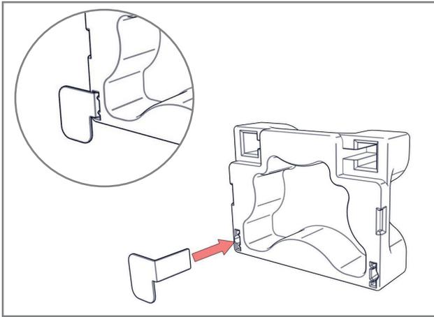
5. Place the bottom corner bracket into the bottom left slot on the bracket fitting tool.
