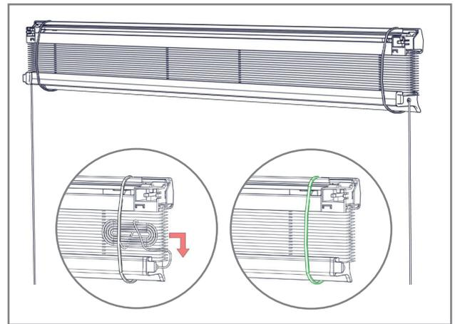
**14.** Remove the cords from the elastic band and allow to hang from the blind. Do not remove elastic bands from the blind.
