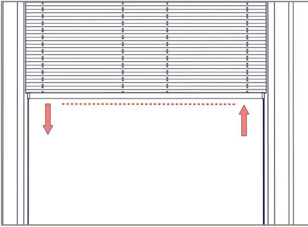
**17.** Cut and remove the elastic bands from the blind. Test the tension by raising the blind, ensure it stays fully raised when released. Ensure bottom bar is straight by adjusting it from side to side.
