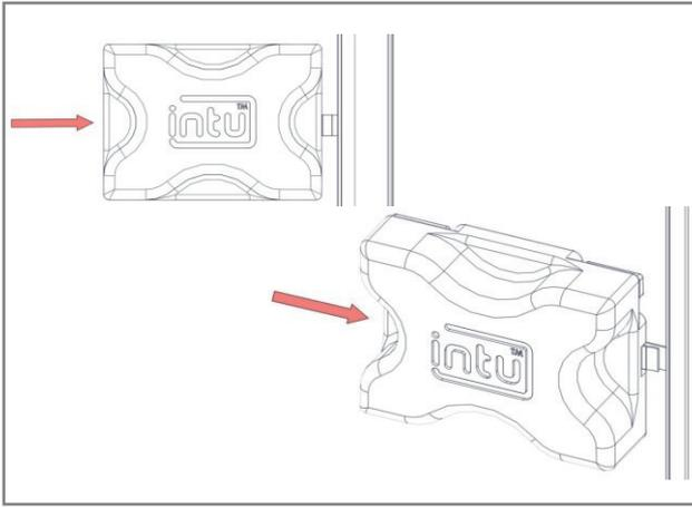
**11.** At the appropriate position(s) on each side profile, fit retention clips (long side profiles only). Press into position using the fitting tool.
