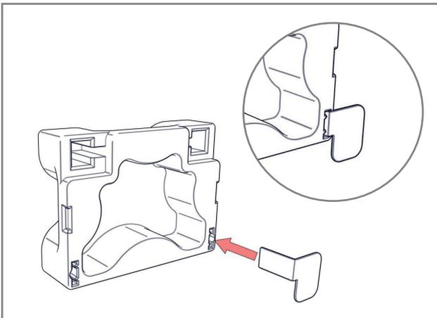
7. Place the bottom corner bracket into the bottom right slot on the bracket fitting tool.
