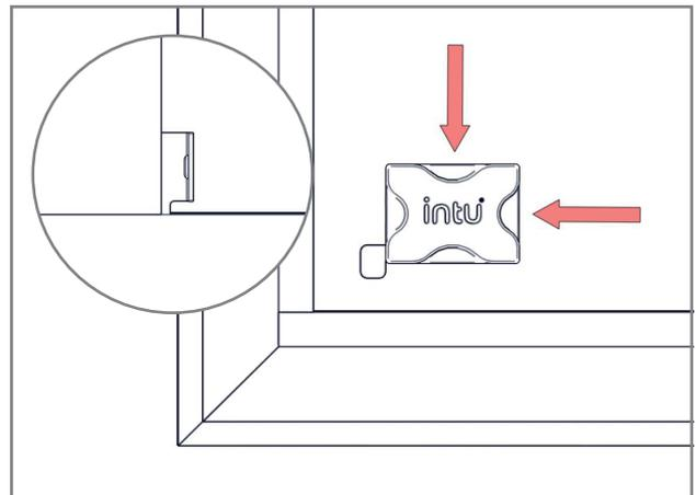
8. Position bracket behind the rubber seal at the bottom right corner of the frame. Carefully push until the metal leg is behind the rubber seal. Check the bracket is square to the sides of the frame and fully secure.
