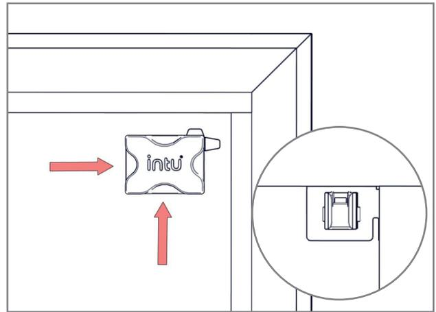
**2.** Position the bracket behind the rubber seal at the top right corner of the frame. Carefully push until the metal legs are behind the rubber seal. Check the bracket is square to the sides of the frame and fully secure.
