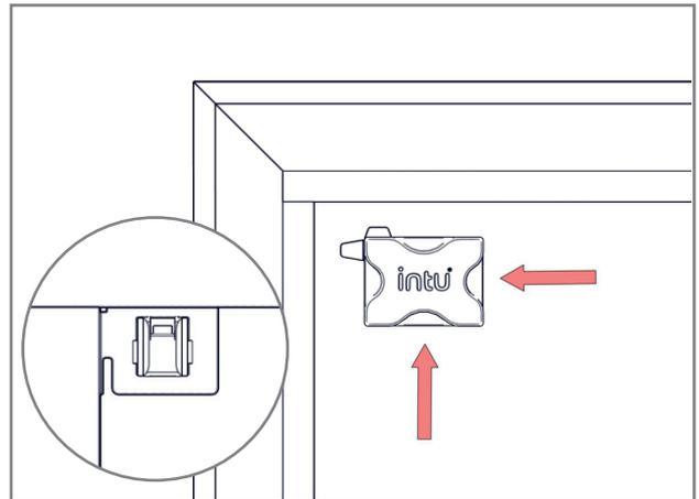
**4.** Position the bracket behind the rubber seal at the top left corner of the frame. Carefully push until the metal legs are behind the rubber seal. Check the bracket is square to the sides of the frame and fully secure.
