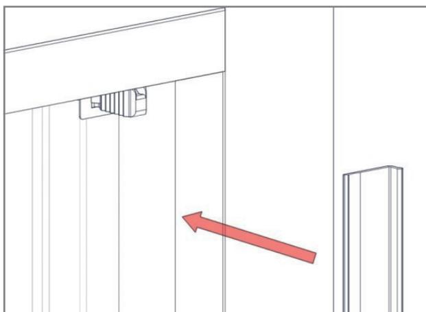
9. Place the flat side of the side extrusion against the glass with the notch to the bottom.
