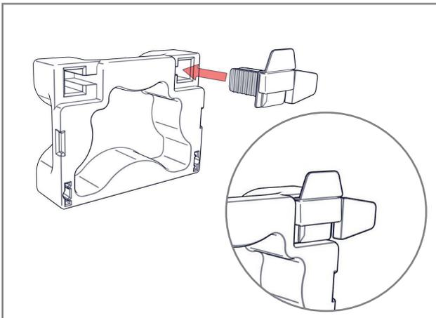
**3.** Place the top corner bracket into the top right slot on the bracket fitting tool.
