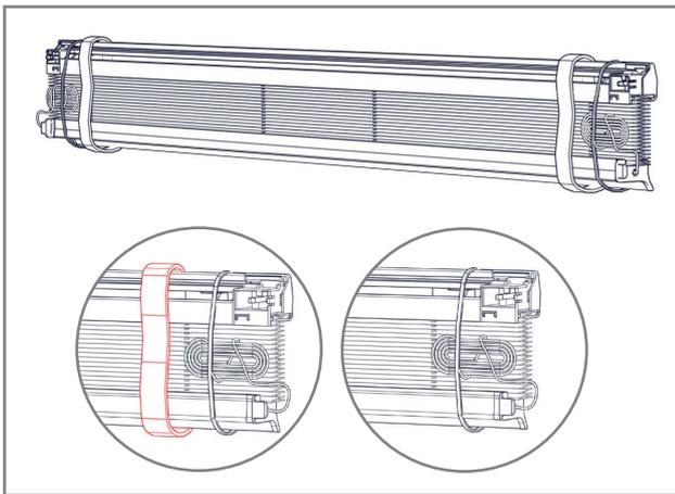
**13.** Remove the Velcro straps that wrap around the blind. Do not remove the elastic bands.
