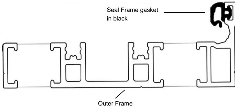
**3** With the frame fully assembled and before installing the frame, fit the Frame Gasket Seal into the frame, as shown on Fig 4.
