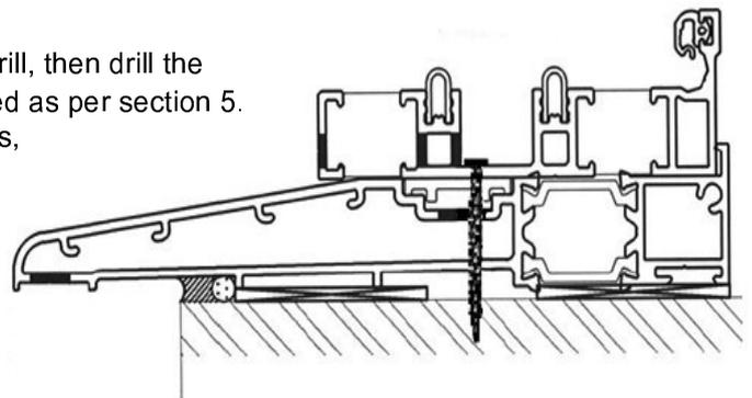
Apply two beads of Silicone between the threshold and cill.
