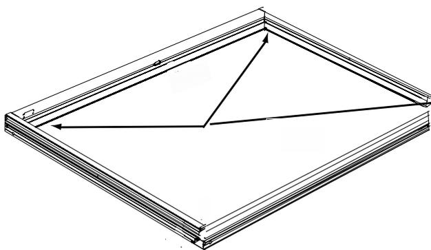
**1** Lay the 4 pcs of frame on the floor on top of cardboard or a similar protective covering to prevent damage to the aluminium.
