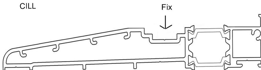
**6c.)** Apply silicone along the length of the Cill paying particular attention to the ends, then lift up the assembled frame and position onto the Cill and swing the frame up into the opening, using packers to hold it in position.
