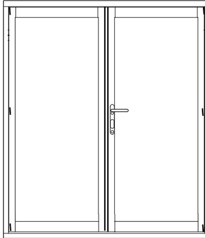
To open the doors, unlock the door with handle by using the key, then depress the handle to open the door.
