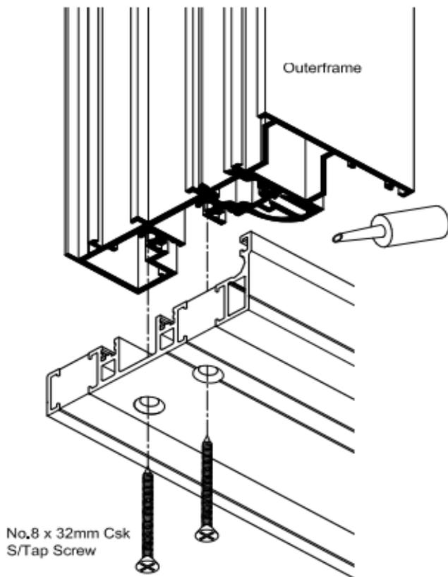
Before locating the jambs onto the bottom rail / track, mastic seal both ends of the jambs and the face of the thermal breaks.
