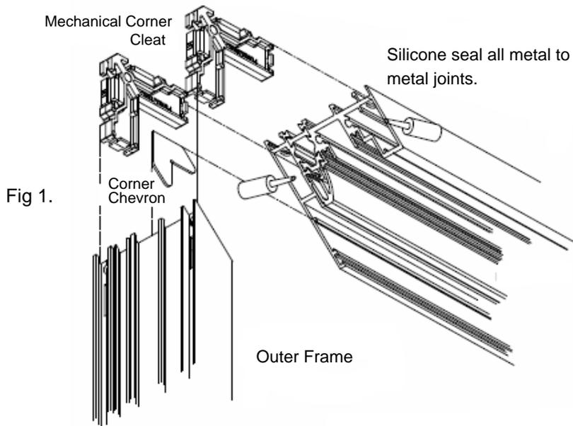
Align the mitred corners and ensure the cleat bullets are in the correct position and fully visible in the slots.
