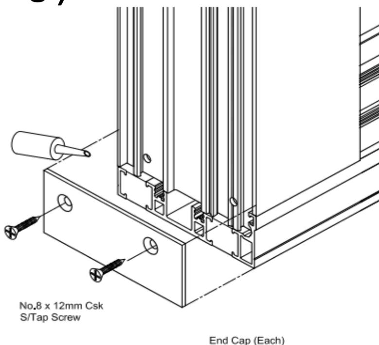
Silicone seal both end caps onto the bottom track / rail to avoid any through drainage using the no.8 x 12mm S/Tap fixing screw.
