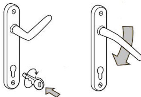
**Unlocking** - turn the key one full turn away from the edge of the door. This disengages the deadlocking security.
