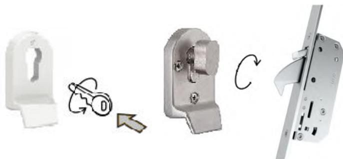
**Unlocking**- From the outside turn the key away from the edge of the door. This disengages the hooks and retracts the latch. The door is then free to open, use the handle to push the door open.
