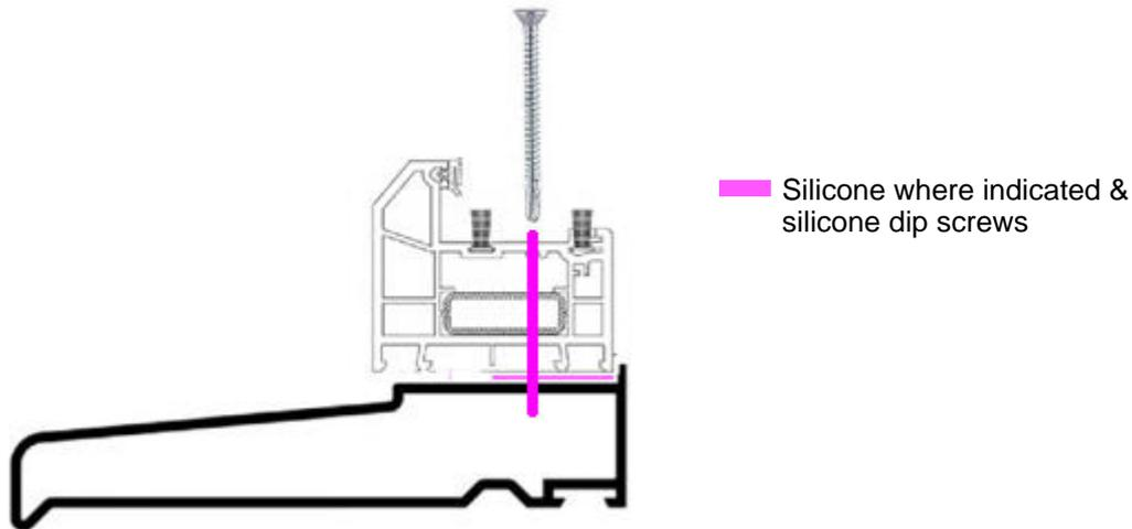
When all the fixing points are loosely secured, check the frame again to ensure it is level in every plane and square in the opening with an equal air gap. Finally, remove any temporary wedges and tighten the fixings, leaving the packers in place, and do one last check with the spirit level.
