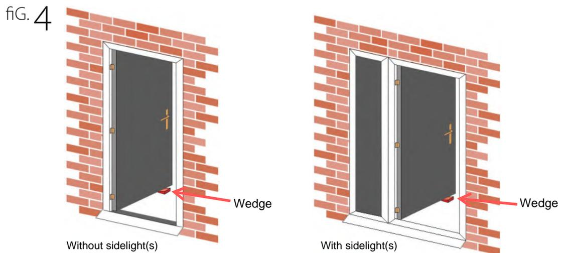
Once you are happy the door set is in correctly, that is with an even air gap all the way round, fix through the outer frame into the brickwork through both jambs, with fixings at spacing shown on Page 7 (figure 5) using the direct frame fixings (A) provided (unless the construction of your building requires more appropriate fixings to suit the individual dwelling).
