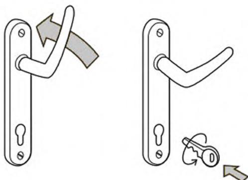
**Locking** - to lock, lift the handle lever in an upwards direction to throw all security bolts. This will engage all locking points into the keeps.
