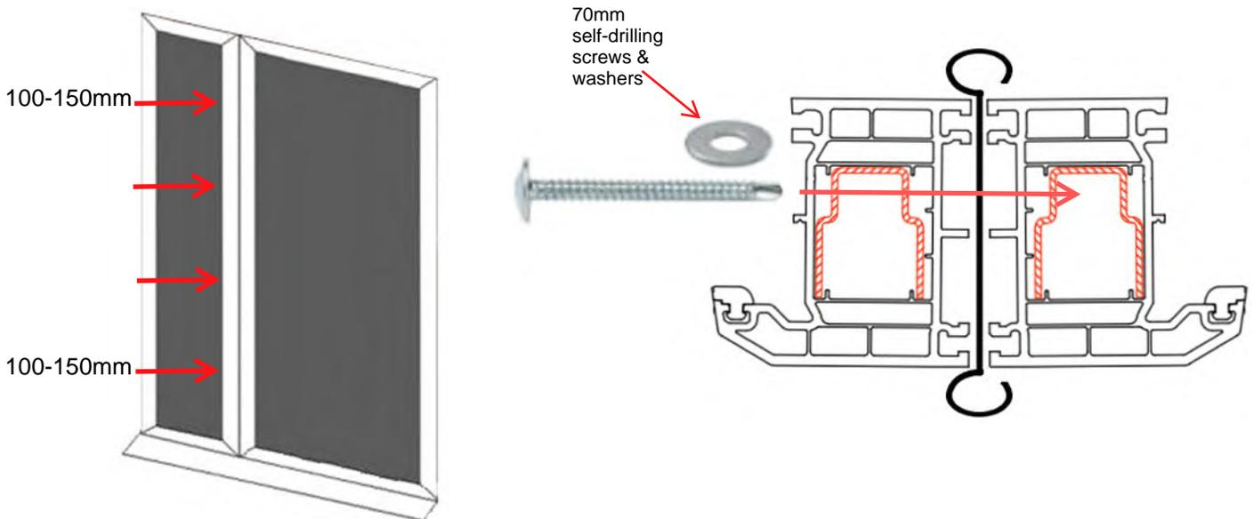
Internal and external trims are supplied to cover the coupler once fully installed.
