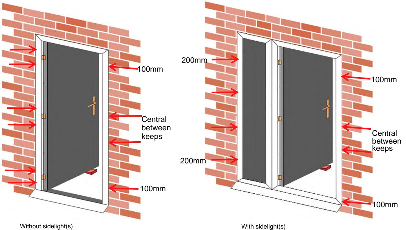
Take care to avoid mortar joints as all fixings need to be secure. Use the direct frame fixings as follows:
