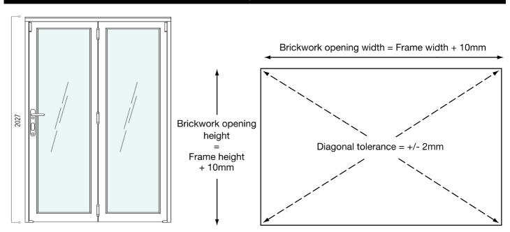
The outer frame height of this door set WITH A THRESHOLD is 2027mm high. The recommended opening height would be + 10mm, i.e 2037mm high.
