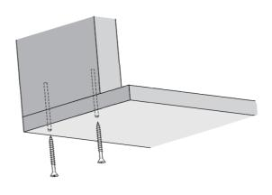
Using the M5 x 70mm wood screws provided attach the threshold to the outer frame jambs.
