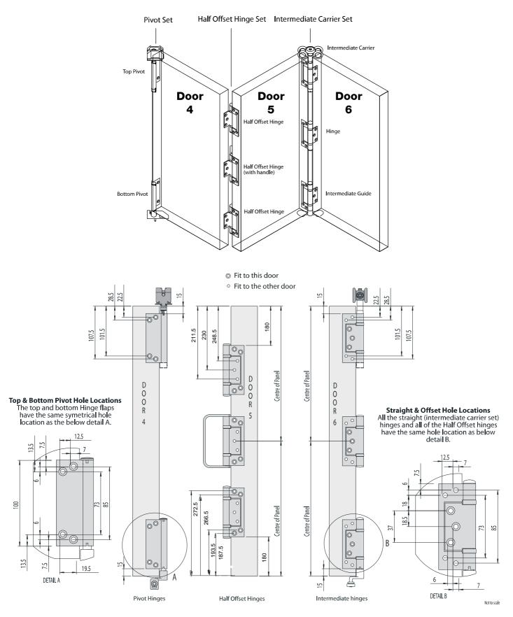
Note: Pivots are reversible. The pivots are delivered set up for this option 'B' - Use without change.
