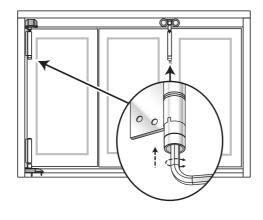
Adjust the top and bottom pivots to move the doors left or right.
