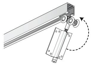
Slide both sets (2) of intermediate carrier wheels into the track.
