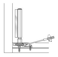
Insert pivot base into cill channel. Drill pilot hole in channel and fix with self-tapping screw.
