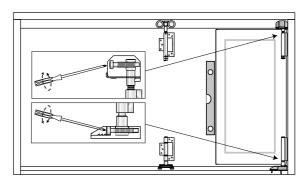
Fit half offset hinges to the inside edge of door 1. Fix through small centre part of hinges using screws provided in pre-drilled holes.
