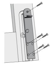
15 Fit the keyed drop bolt cups to the cill in the pre-cut positions.
