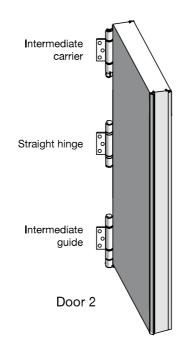
Lift door 2 and locate intermediate guide in bottom channel. Support door on blocks then screw top carrier bolt into top wheel assembly.
