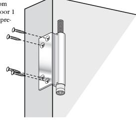
Assemble top pivot block. Slide and click cover plate onto the pivot block. Screw through cover plate into rear of access slot ensuring the pivot block is sitting tight up against the frame jamb.
