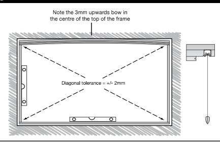
10 Fix the outer frame into the brickwork, setting it to overbang the cavity. Install sill onto a bed of silicone sealant and/or mortar.
