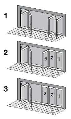
**36** When closing the right door set, first close doors 1 and 2, securing them with the dropbolts. Then close door 3. When closing the left door set, first close doors 4 & 5, securing them with the dropbolt. Finally, close and lock door 6.
