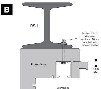
The aluminium top track, which is temporarily held in place with transit screws, has been pre-drilled for fixing points into the Lintel.
