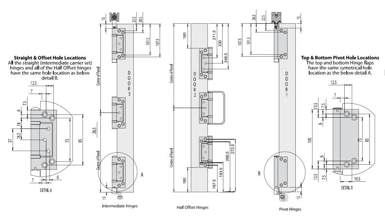
Note: Pivots are reversible. For this option 'A' it is necessary to take the top and bottom pivots apart to reverse them - see 16
