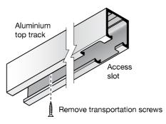
$6 \quad \begin{array}{ll} \text{Remove the two transportation screws} \\ \text{to release the aluminium top track} \\ \text{from the frame head.} \end{array}$
