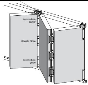
Drawings in this section show the arrangement of parts for Opening Option
