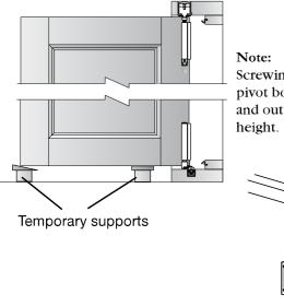
Screwing top pivot bolt in and out adjusts
