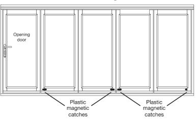
**39** When closing the door set, first close doors 1 and 2, securing them with the dropbolts. Then close doors 3 and 4, securing them with the dropbolts. When opening and closing the doors ensure the access door (door 5) is in the open position and closes last, otherwise the access door will catch on the cill.
