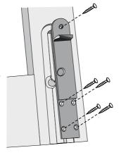
15 Fit the keyed drop bolt cups to the cill in the pre-cut positions.
