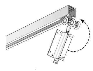
7a Slide the intermediate carrier wheels into the track.
