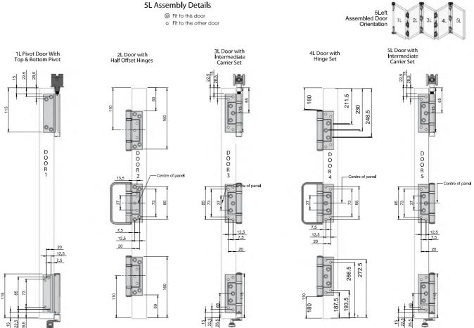
Note: Pivots are reversible. The pivots are delivered set up for this option 'B' - Use without change.
