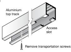
6a Remove the two transportation screws to release the aluminium top track from the frame head.
