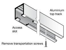
Remove the two transportation screws to release the aluminium top track from the frame head.
