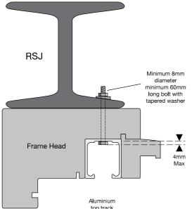
The aluminium top track, which is temporarily held in place with transit screws, has been pre-drilled for fixing points into the Lintel.
