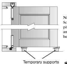
Note: Screwing top pivot bolt in and out adjusts height.
