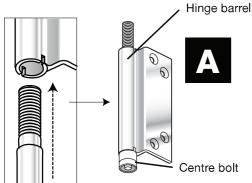
17 Fix top and bottom pivot hinges to door 1 using screws supplied in predrilled holes
