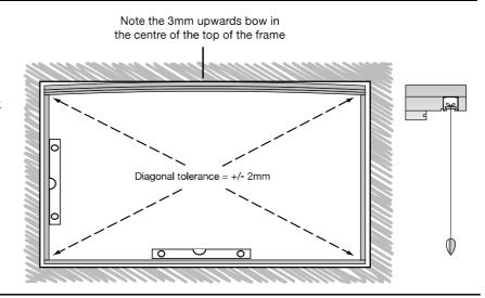
10 Fix the outer frame into the brickwork, setting it to overbang the cavity. Install sill onto a bed of silicone sealant and/or mortar.
