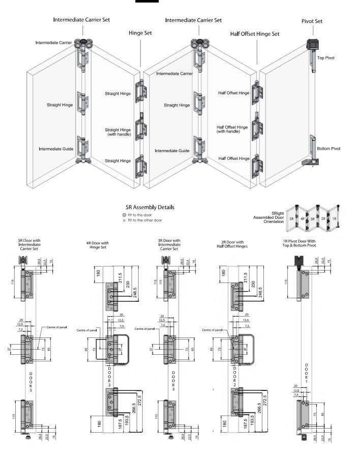
Note: Pivots are reversible. For this option 'A' it is necessary to take the top and bottom pivots apart to reverse them - see 16
