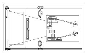
Fit half offset hinges to the inside edge of door 1. in the machined position using screws provided.
