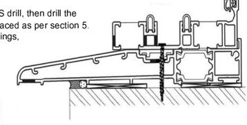
Apply two beads of Silicone between the threshold and cill.
