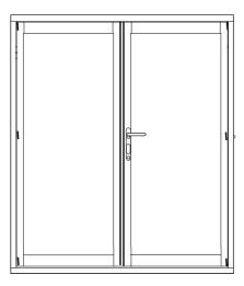
To open the doors, unlock the door with handle by using the key, then depress the handle to open the door. To open the slave door, pull the handle in the edge of the door, to dis-engage the twin point lock. Both doors can then be fully opened.
