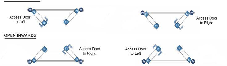
The frame and doors are exactly the same for BOTH open inwards and open outwards.
