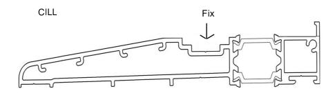
Apply silicone along the length of the Cill paying particular attention to the ends, then lift up the assembled frame and position onto the Cill and swing the frame up into the opening, using packers to hold it in position.
