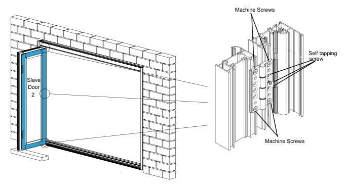
**b** •) With the door at right angles and supported on blocks (being careful not to damage the seal on the bottom of the door). Use the 2pc Allen key Head machine screws and 3pc self tapping screw to secure each hinge leaf.
