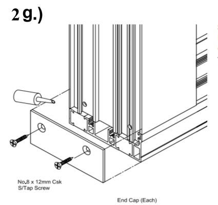
Silicone seal both end caps onto the bottom track / rail to avoid any through drainage using the no.8 x 12mm S/Tap fixing screw.
