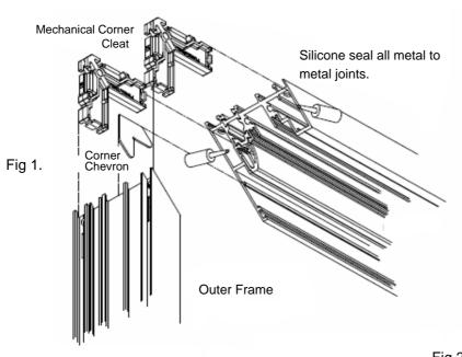
Align the mitred corners and ensure the cleat bullets are in the correct position and fully visible in the slots.
