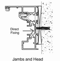
Direct fix 150mm from all corners and every 600mm maximum centres, using the hardened steel frame fixings provided.
