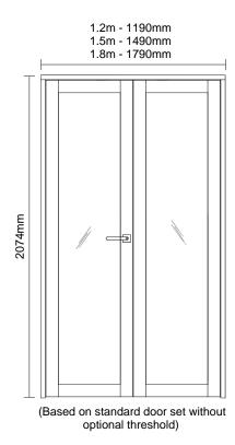
Brick / stud work opening = Frame width + 10mm
