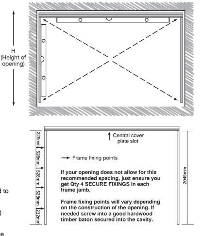
Very important: Carefully check the frame is tightly fixed together and is square. Diagonals of the frame must be equal. Do not proceed with installation if the frame is not square.
