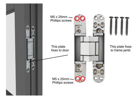
With a second pair of hands to steady the door, or with the door packed up on blocks / discarded packaging, fix the hinge plate to the door with the M5 x 25mm Phillips screws and PH2 drill bit (F) supplied, Qty 4 per hinge plate. Careful not to round off the screw heads, use a low driver setting.
