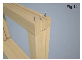
Fixing frame jamb to head
