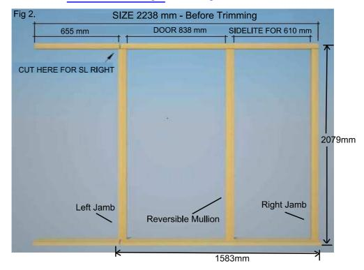
Assembled outer frame size: 2079mm High x 1583mm Wide Brick work OPENING size: 2089mm High x 1593mm Wide
