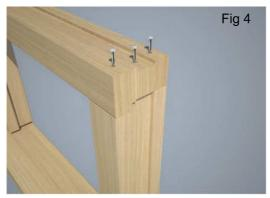
Fixing frame jamb to head
