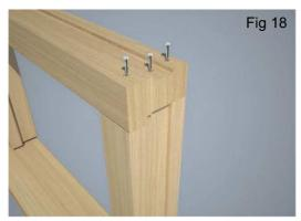
Fixing frame jamb to head
