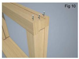
Fixing frame jamb to head
