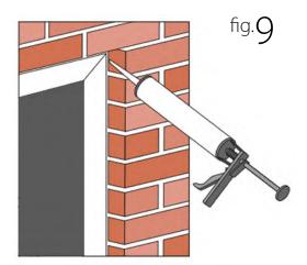
Seal under and around the outside of the cill, ensuring you do not block any of the drain holes.
