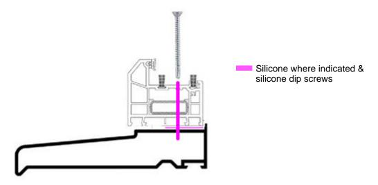
When all the fixing points are loosely secured, check the frame again to ensure it is level in every plane and square in the opening with an equal air gap. Finally, remove any temporary wedges and tighten the fixings, leaving the packers in place, and do one last check with the spirit level.
