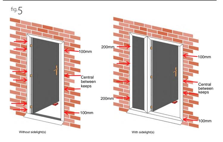
Take care to avoid mortar joints as all fixings need to be secure. Use the direct frame fixings as follows:
