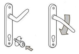
**Unlocking** - turn the key one full turn away from the edge of the door. This this disengage the deadlocking security.
