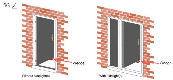
Once you are happy the door set is in correctly, that is with an even air gap all the way round, fix through the outer frame into the brickwork through both jambs, with fixings at spacing shown on Page 7 (figure 5) using the direct frame fixings (A) provided (unless the construction of your building requires more appropriate fixings to suit the individual dwelling).
