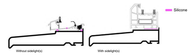
IMPORTANT the frame should not be pushed tight back to the plaster line as this can lead to the door being fitted in twist.
